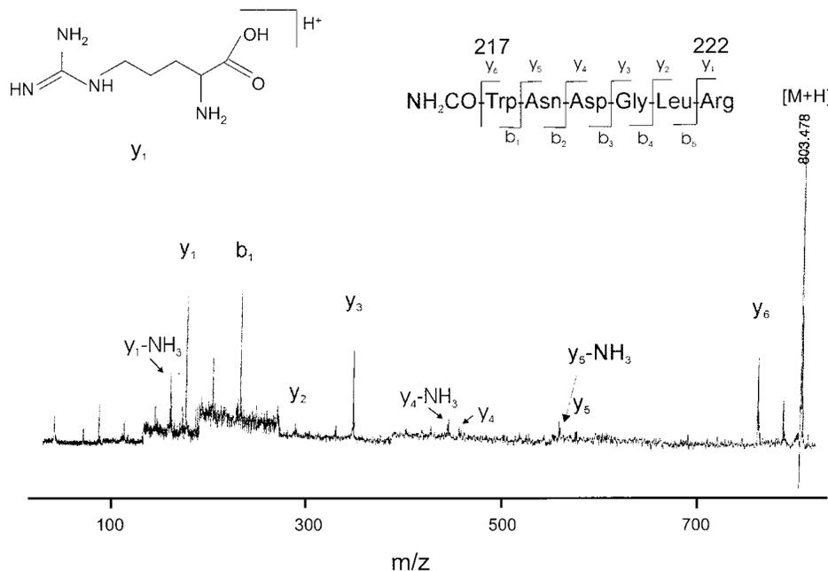
**Fig. 3.** MALDI-PSD analysis of tryptic peptide fragment N-carbanoyl-ScrY (217–222). Signal of sequence-specific fragments  $y_1$ – $y_6$  and corresponding fragments by loss of  $\text{NH}_3$  are denoted; b-ions (except  $b_1$ ) and other fragments are not denoted.
