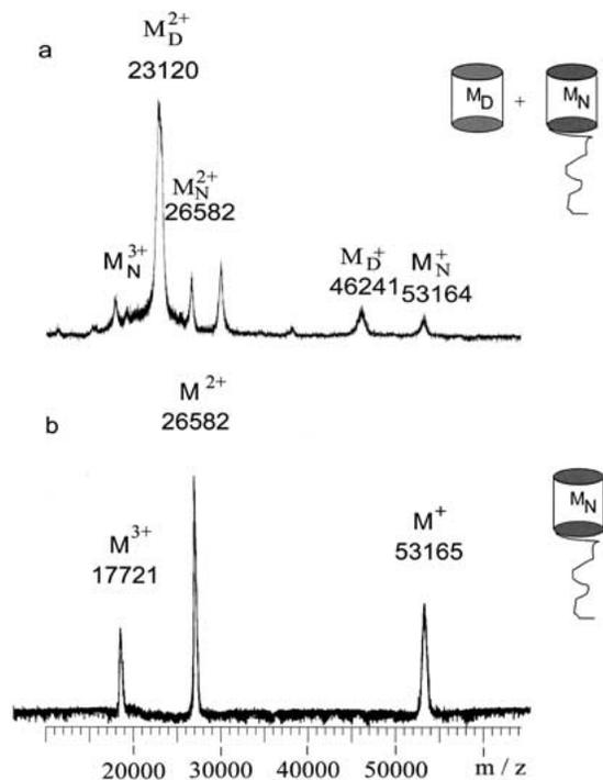
**Fig. 2.** MALDI-MS analyses of (a) intact ScrY porin and (b) partially truncated ScrY-tr. Spectrum a was obtained in 0.04% dodecylmaltoside, spectrum b in 0.15%  $\beta$ -octylglucoside as described in Materials and Methods. The  $\beta$ -barrel scheme  $M_N$  indicates full-length intact ScrY (M.W. = 53164 daltons),  $M_{tr}$  indicated the truncated ScrY (M.W. = 46240 daltons).
